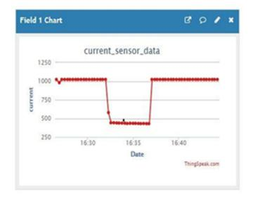
Fig. 4. Screenshot of energy meter current consumption data by electrical load
